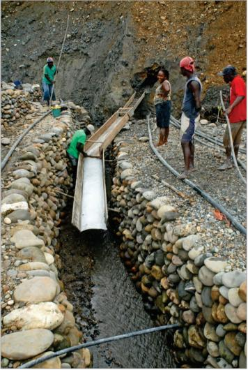
Artisanal mining method performed by Afro-Colombian communities where sands are washed utilizing water presure. Ponds, gravety and ocassionally small water pumps are utiled for creating pressure. Photograph by Oro Verde.
